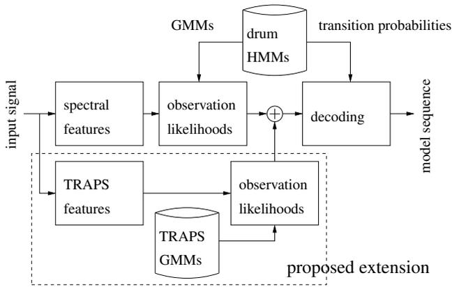
**Figure 2.** Block diagram of the full system with the proposed extension circled with dashed line.
