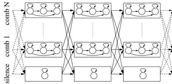
**Figure 3.** The idea of the used HMM model network consisting of drum combinations (“comb 1” and “comb N”) and the silence model.
